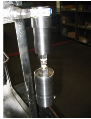
External coalescing filter option Ensures clean/dry air/gas
